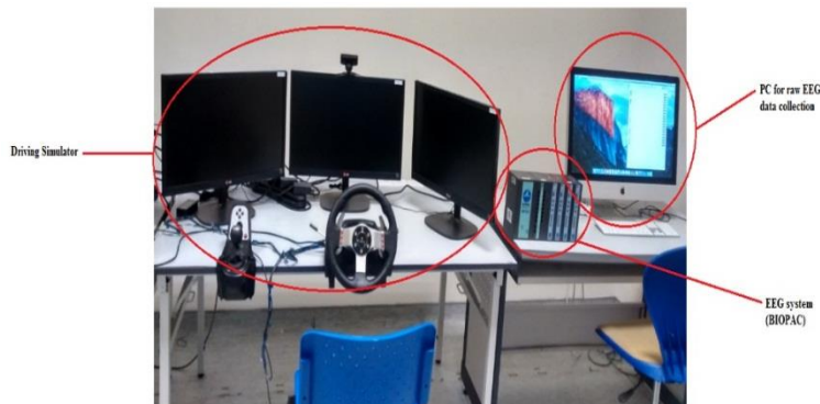
Fig. 3. Design of apparatus for in-lab experiment purpose.
