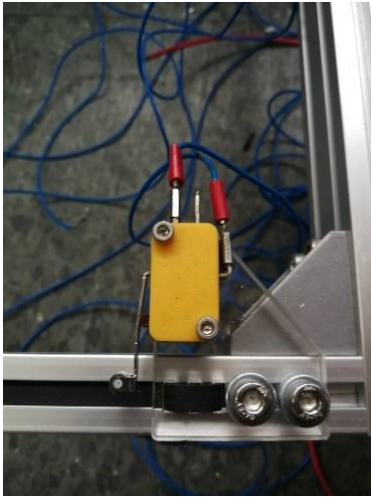
Fig. 8. Installation of limiting switch.
