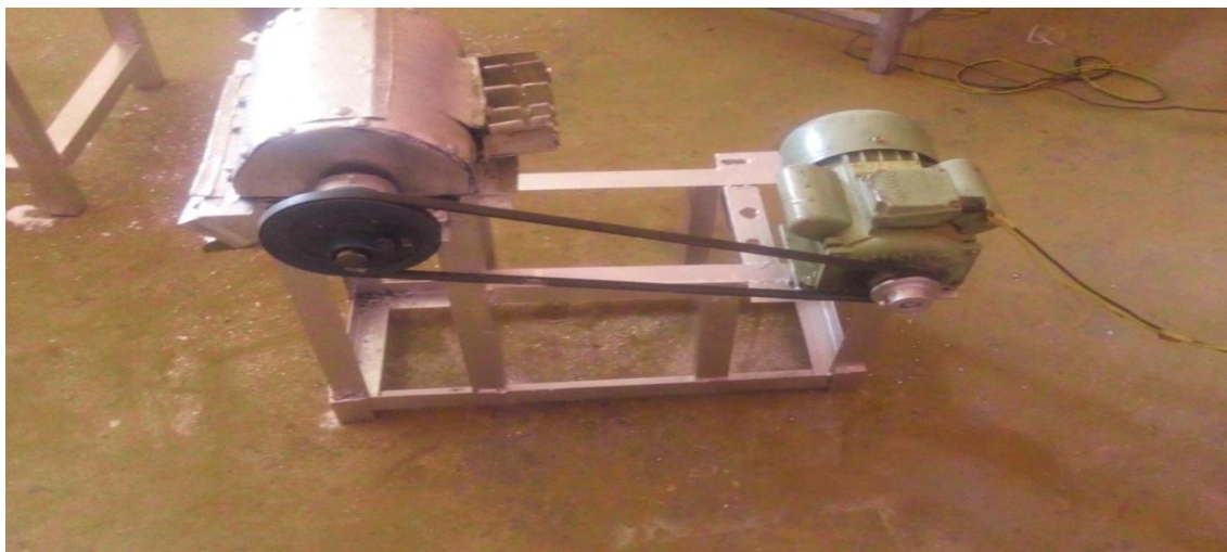
Plate 1: Small Scale Okro Slicing Machine.
