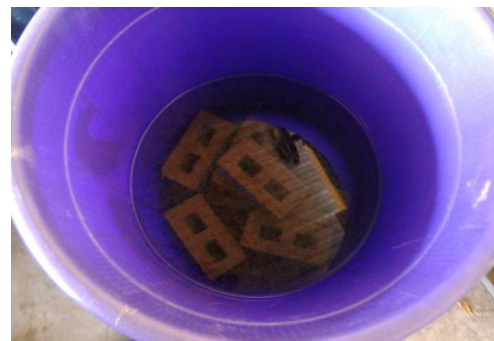
Figure 4: Hollow masonry unit under curing
