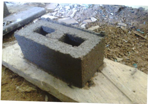
Figure 3: Freshly moulded hollow block
