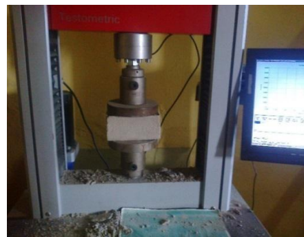
Figure 5: Masonry unit under compressive test
