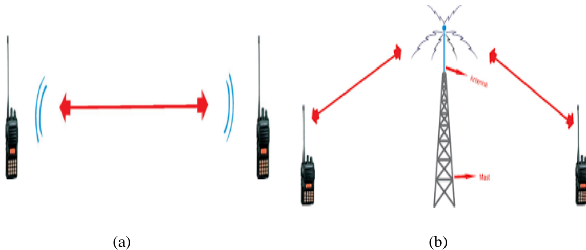
Figure 5: Two-way radio system (a) Repeater operation (walki-talkie) and (b) Using base station (infotrunk, 2016)
