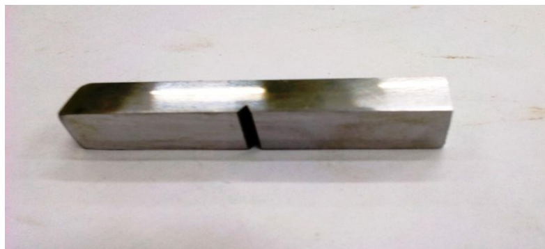
Figure 3: Charpy test specimen
