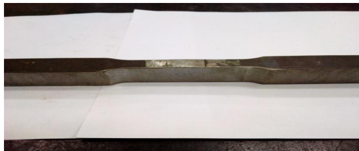
Figure 1: Tensile test specimen
