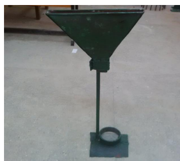
Figure 2.2: Set up for Flow ability of Mortar (Mini-V-Funnel).
