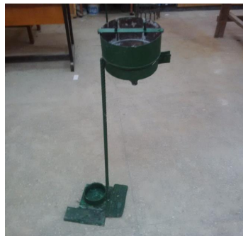
Figure 2.1: Set up for Filling ability (Flow Cone Test).
