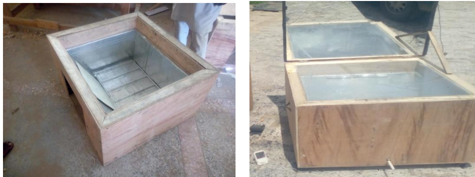
Figure. 4: Box unit with PCM tank before and after glazing
