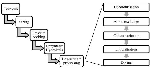
Figure 1. General manufacturing steps of XOS from corn cob.
