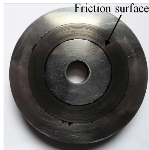
Fig. 9 – Thin layer on the contact surface of the pin (Ep/Ca/Oil) on disc
