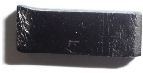
Fig. 7 – A sample Ep/Ca/Oil deformed during a wear test at 3Mpa.m/s
