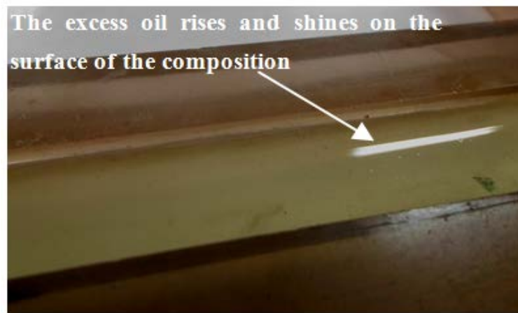
Fig. 2 – Excess oil rises to the surface after polymerization of the composition Ep/Oil
