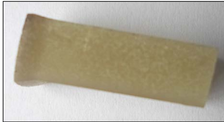
Fig. 6 – A sample Ep/Oil deformed during a wear test at 1Mpa.m/s
