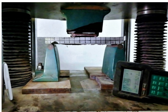
(c) Test setup of flexural strength test
