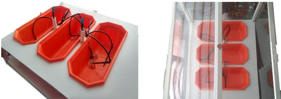
Figure 12. Moist, humidity and temperature sensors, hoses and stakes (left), Light sensor (right).
