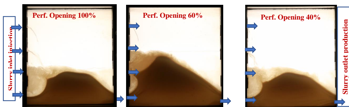
Figure 8. Real picture of experiment results shown perforation opening size effect on proppant transport, perf opening 100% (left), perf opening 60% (middle) and perf opening 40% (right).
