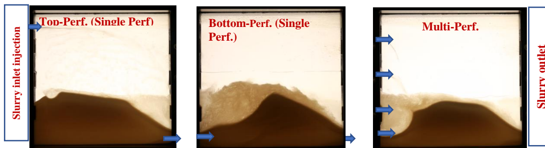
Figure 5. Real picture of experiment results shown number of perforation effect on proppant transport, Top-perf (left), Bottom-perf (middle) and Multi-perf. (right).
