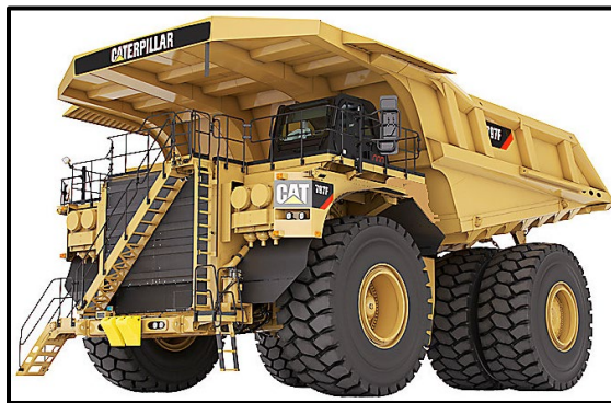
Figure 3.1 CAT 797F conventional rear dump truck [166]
