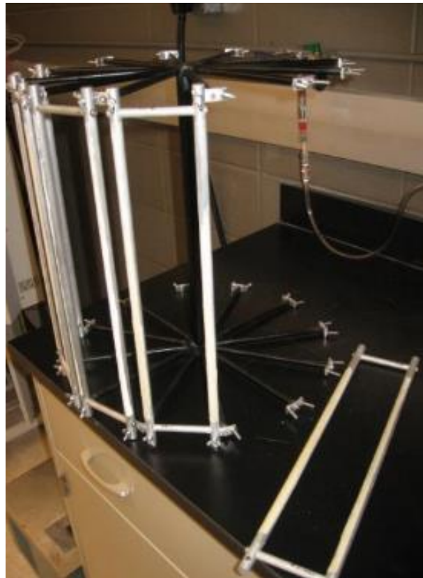
Figure 2.4. The removable frame cage for fiber pulling.
