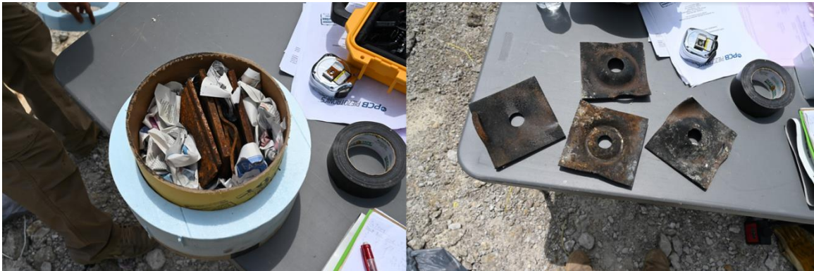
Figure A.39. Roof bolt plates
