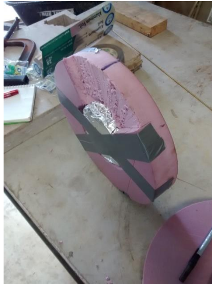
Figure 2.4. Black powder charge construction
