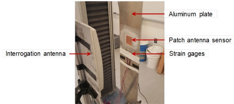
Fig. 3-25 Experimental setup for tensile testing
