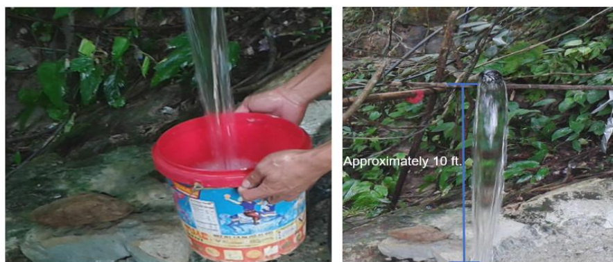
Figure 6. Actual testing of the volume flow rate of the source (left) and height of the drop of the source (right).
