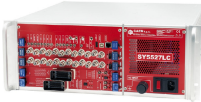
Figure 5.32: The HV CAEN sy5527 provide power supplies to PMTs of Local Monitor system.
