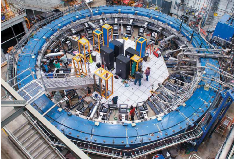
Figure 4.3: The E821 ring magnet in the MC-1 building at Fermilab. Courtesy of Fermi National Accelerator Laboratory.
