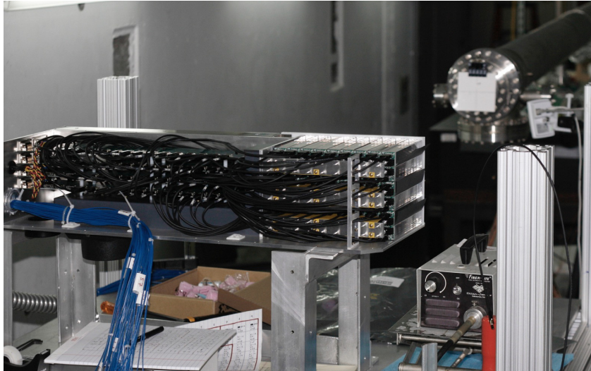
Figure 6.10: Calorimeter sitting on top of the table at SLAC. The electron beam is coming from the long tube is heading towards here.
