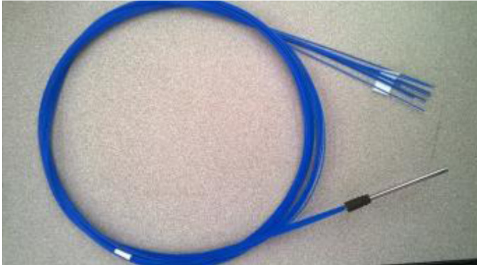
Figure 5.22: Mini bundle of fibers drives the light collected by the Source Monitor to Local Monitors. Are used 6 mini bundles, each used for 1 SM and 4 LM are used.
