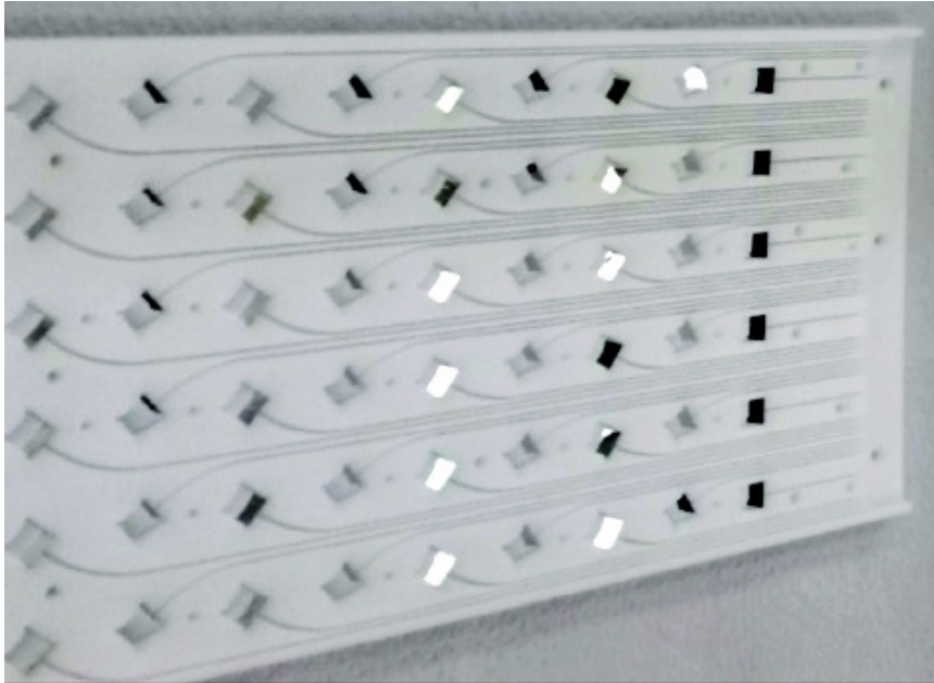
Figure 5.15: Picture of the front panel. Each hole in the delrin plate house a 5 mm 45^\circ prism which deflects the light coming from the fiber placed inside the groove.
