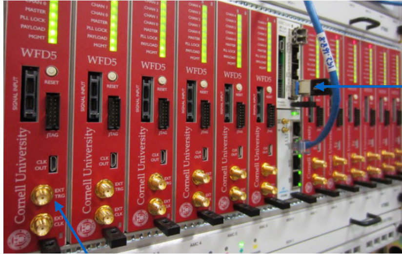
Figure 4.15: \mu TCA with 12 waveform digitizers, part of DAQ system used in g - 2 experiment at Fermilab.
