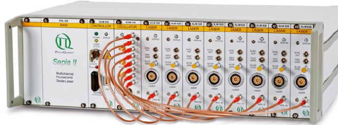
Figure 5.30: Laser crate “Sepia”. Each laser head LDH-P-C-405M will be coupled to its driver (the crate contains up to 8 drivers).
