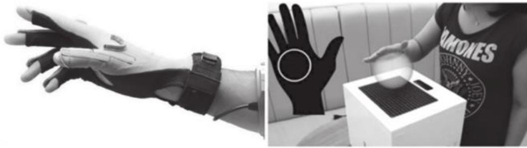
Figure 5: Sensing Gloves and Computer Motion Capture Recognition
