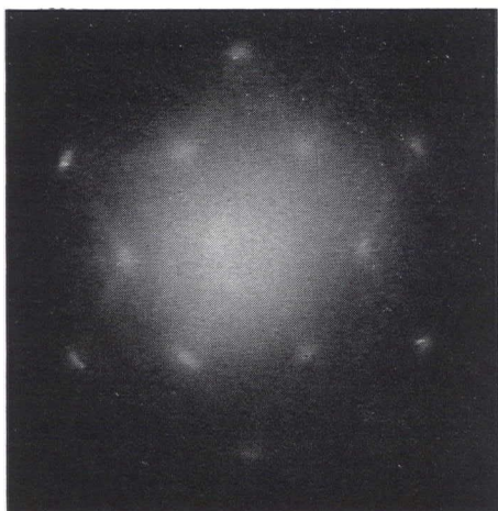
Figure 5 Selected area electron diffraction pattern of a single platelet crystal of alpha iron.
