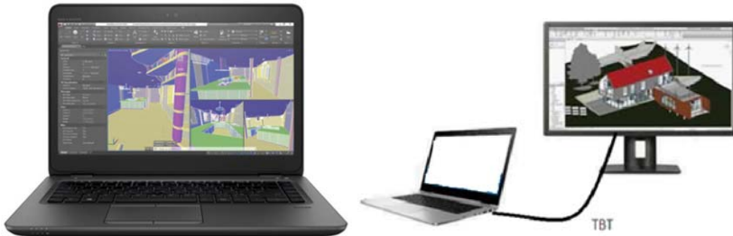
Figure 1. An TBT eGFX display allows user can use smaller notebook have good graphic progress ability when connecting to TBT eGFX monitor.
