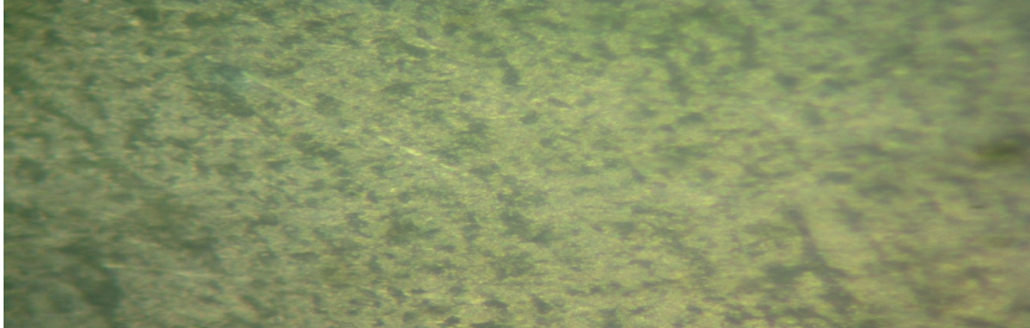
Figure 7: Micrograph of RPE matrix reinforced with 5wt%PKSA of 100 \mu m particle size
