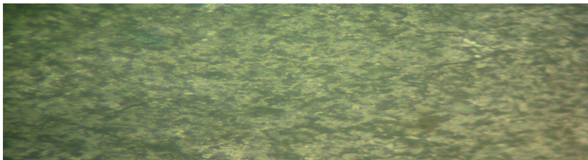
Figure 9: Micrograph of RPE matrix reinforced with 20wt%PKSA of 100 \mu m particle size
