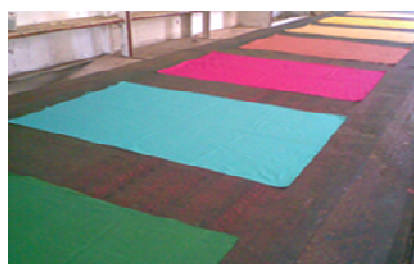
Fig. 2b: Samples stretched on table ready for printing.
