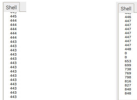
Fig 7a: Correct 3.3 Volt CO 2 Sensor Measurement Fig 7b: 5.5 Volt Inflated CO 2 Sensor Measurement
