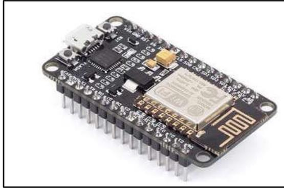
**Figura 5-1:** NodeMCU
