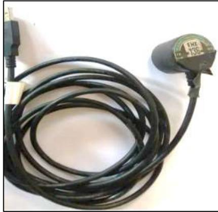
**Figura 7-2:** Sonda Óptica USB
