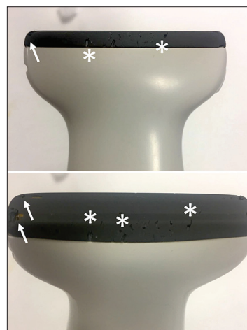
Figure 1: Ultrasound damaged probe
