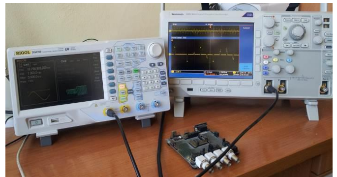
Fig. 6. Devices in the laboratory (function generator Rigol DG4102 and oscilloscope Tektronix DPO3012) together with FPAA circuit.
