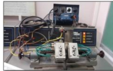
Figure 3. FG HAZ specimens prepared in welding simulator
