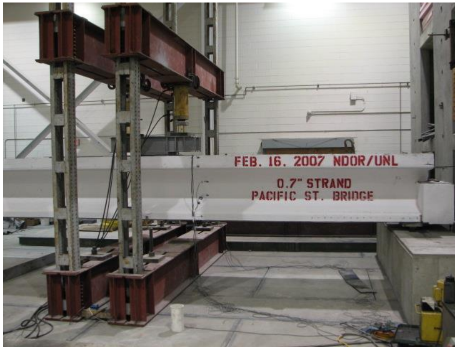
Figure 10. Load testing of NU900 girder
