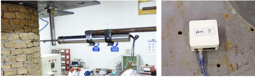
Figure 14. The LVDT and accelerometer
