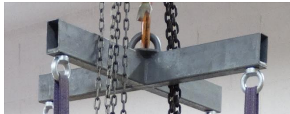
Figure 8. Steel bars with four hooks
