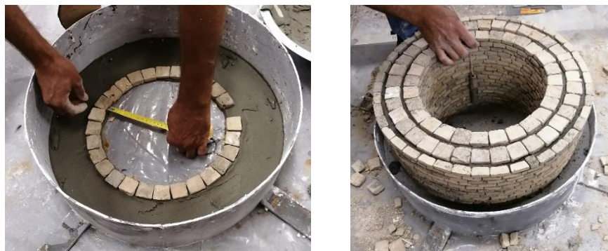
Figure 9. Checking the dimensions and the alignment during the model construction
