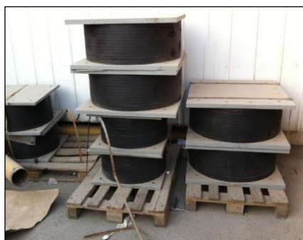
Figure 1. Lead-rubber bearings with different dimension
