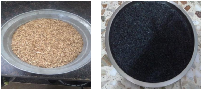
Figure 1. Raw rice husk before and after burning
