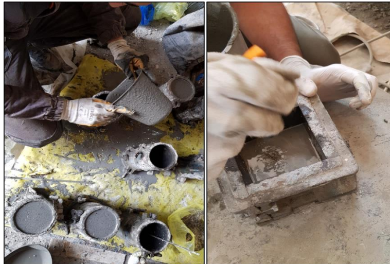
Figure 4. Pouring processes of SIFCON samples
