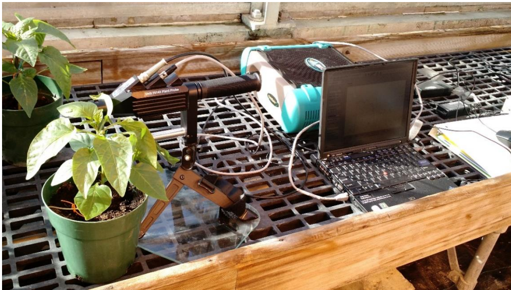
Figure 9. Field hyperspectrometer, laptop and leaf clip while performing a measurement.
