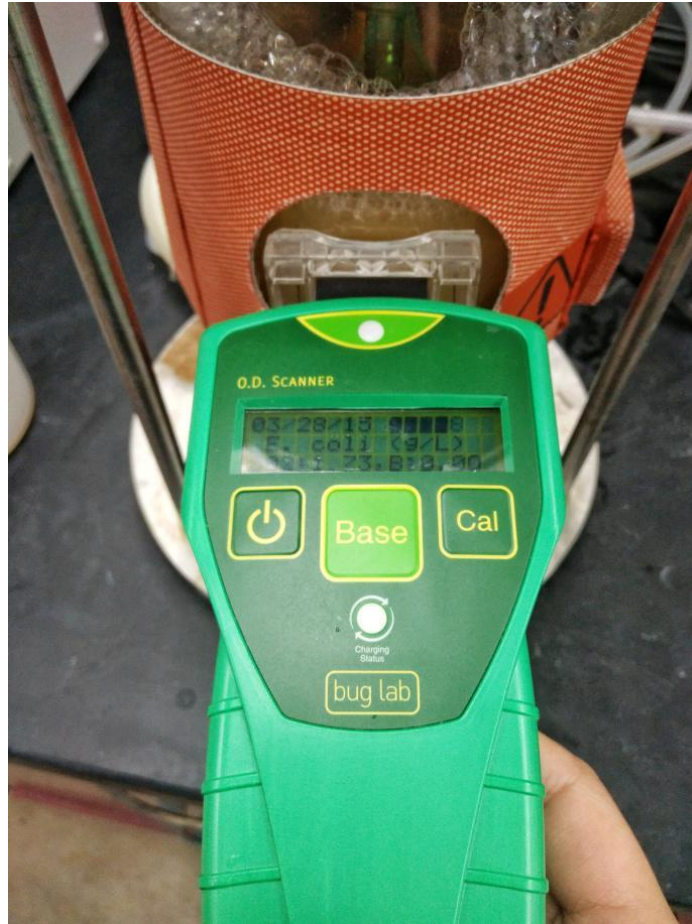
Figure 3.5 The OD scanner used for determination of cell biomass concentration located at lab 204 of department of Paper and Bioprocess Engineering, SUNY-ESF.
