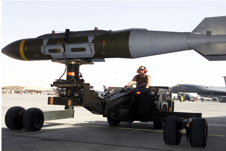
Figure 1: Bomb equipped with the JDAM tail package being loaded into the bomb bay of a B-1 Lancer (Source: Military.com)
