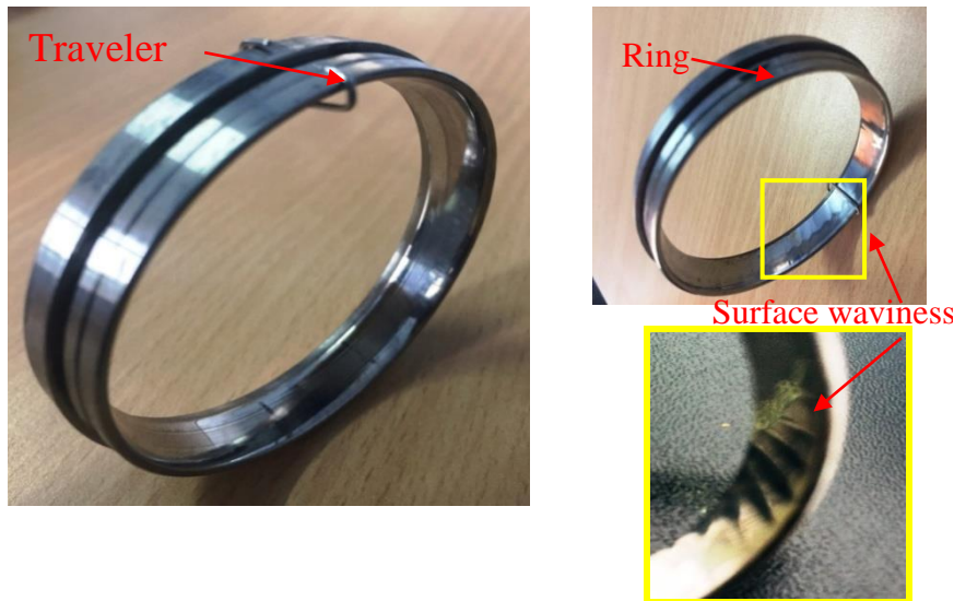
Fig. 1 New spinning Ring (left) and damaged Ring surface (right)
