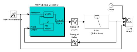
Figure 6. Simulation of Network Closed-Loop Control System based on Predictive Neural
