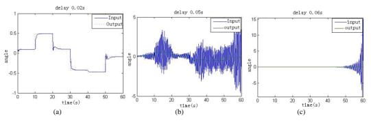
Figure 2. The Influence on the Stability of the Control System from Remote Control Delay
