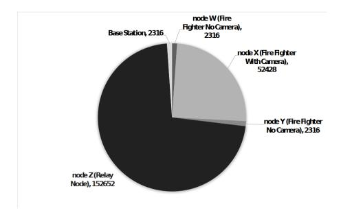
Figure 16: Bit allocation for a 5 node communications mesh with some nodes transmitting commpressed images.
