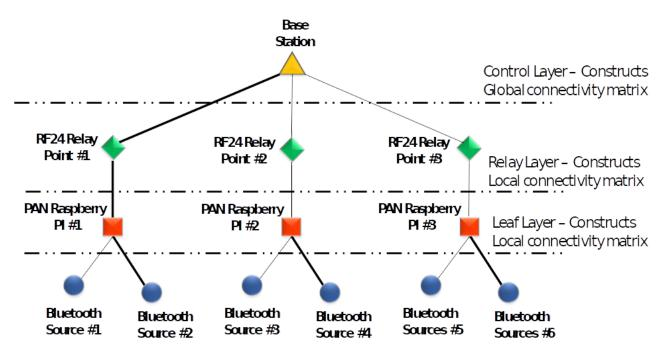
Figure 5: Example of data flow diagram of the mesh network
