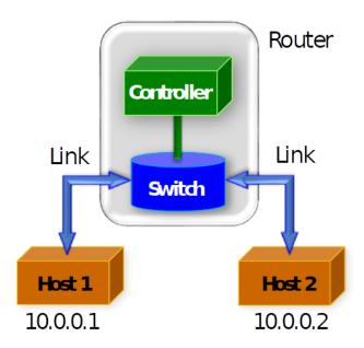
Figure 18: *Mininet* uses 4 components (hosts, links, switches, and controllers) to represent an Eithernet network.
