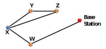
Figure 13: Typical degraded network topology.
