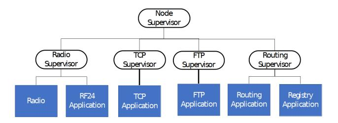
Figure 8: Node supervisor structure.
