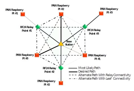
Figure 6: Maximum Interconnectivity Schematic – Note multiple instances of PAN nodes were used to simplify the drawing. So, all nodes labelled PAN Raspberry PI # 1 are the same physical location.
