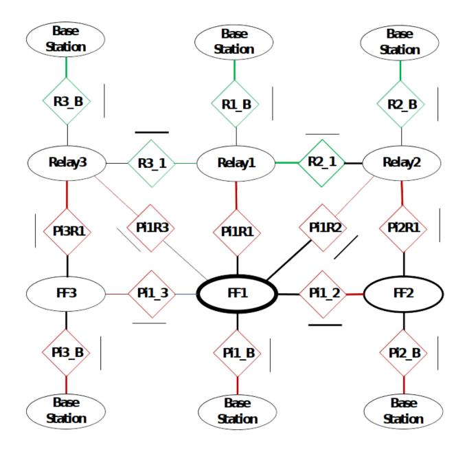
Figure 20: Mininet Topology for a fire fighter node sending data to the base station.
