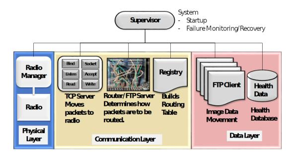
Figure 7: Figure 3. Communication node structure.
