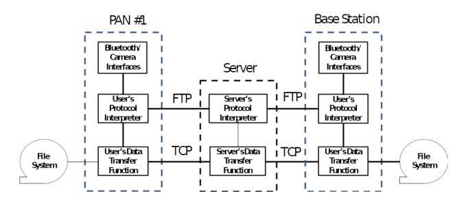
Figure 17: Figure 13 FTP file transfer mechanism
