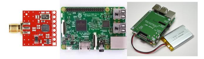
Figure 4: Hardware used for the fire fighter nodes and the relay points to be placed as standalone transceivers.
