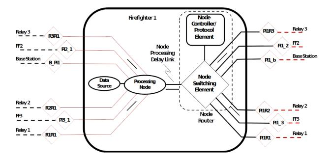
Figure 21: Mininet Firefighter node Topology.
