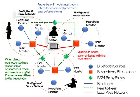
Figure 1: System schematics of the deployed fire fighter communications prototype. Blue dots are the different sensors including a SCBA monitor and others. They are copnnected via Bluetooth to the single board computers (red squares), which connect with the resto of boards using a radio module. Thermal cameras are assumed to be wired to the board. The green diamonds are single board computers endowed with a radio that act as additional relay nodes and they can be left in strategic positions.
