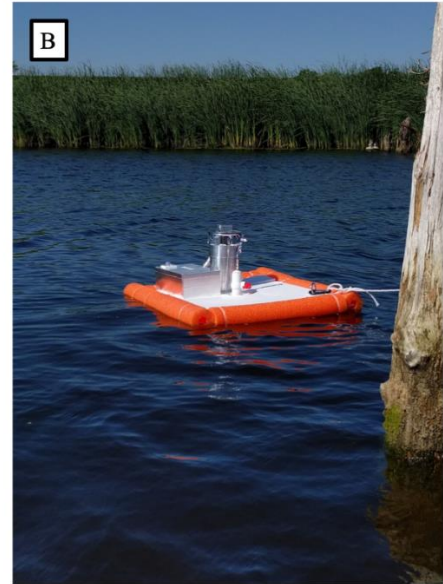
Figure 2.5: Conceptual diagram of automated ebullition sensor validation experiment (A); and photo of AESv2 deployed in the field in the South Tobacco Creek Watershed, Manitoba, Canada (B).
