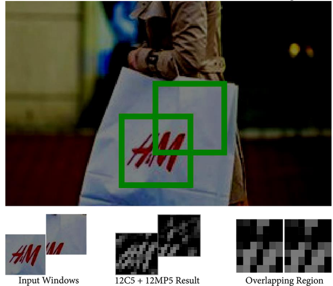
Fig. 4. Two adjacent windows extracted from an input image, passed through the 12C5 + 12MP5 feature extractor. A detailed view of the convolved maps in the overlapping top-right and bottom-left quarters of each window shows that these areas fully match.
