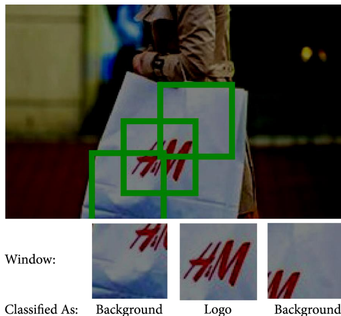
Fig. 3. An overview of the sliding window method, where an input image is subdivided into smaller overlapping image patches, each being individually analyzed by a CNN. A classification result is then obtained for each
