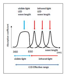
Fig. 7. Light absorption wavelengths of optical multilayer.
