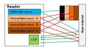
Fig. 6. Principle for reading an optical information medium.
