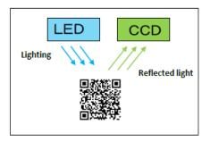
Fig. 4. Principle for reading an optical information medium.
