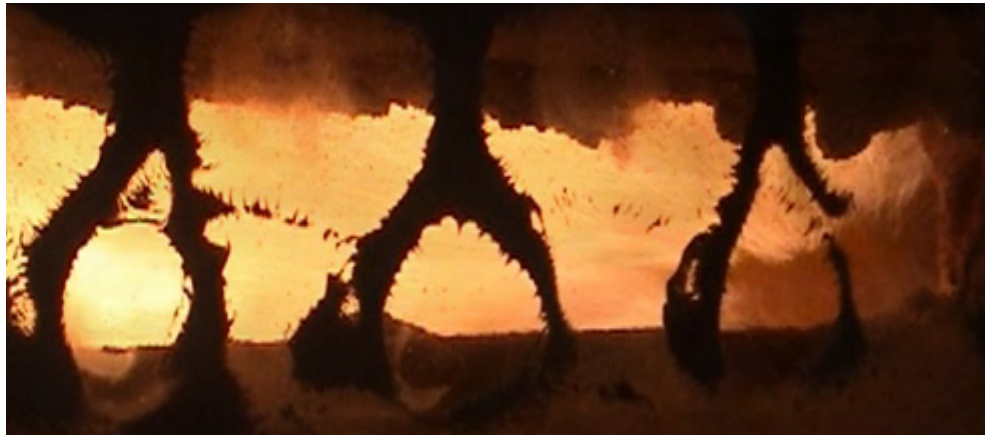
Figure 5.36: Test 98 – “normal conditions”, secondary air flow: 160 \text{ Nm}^3/\text{h}
