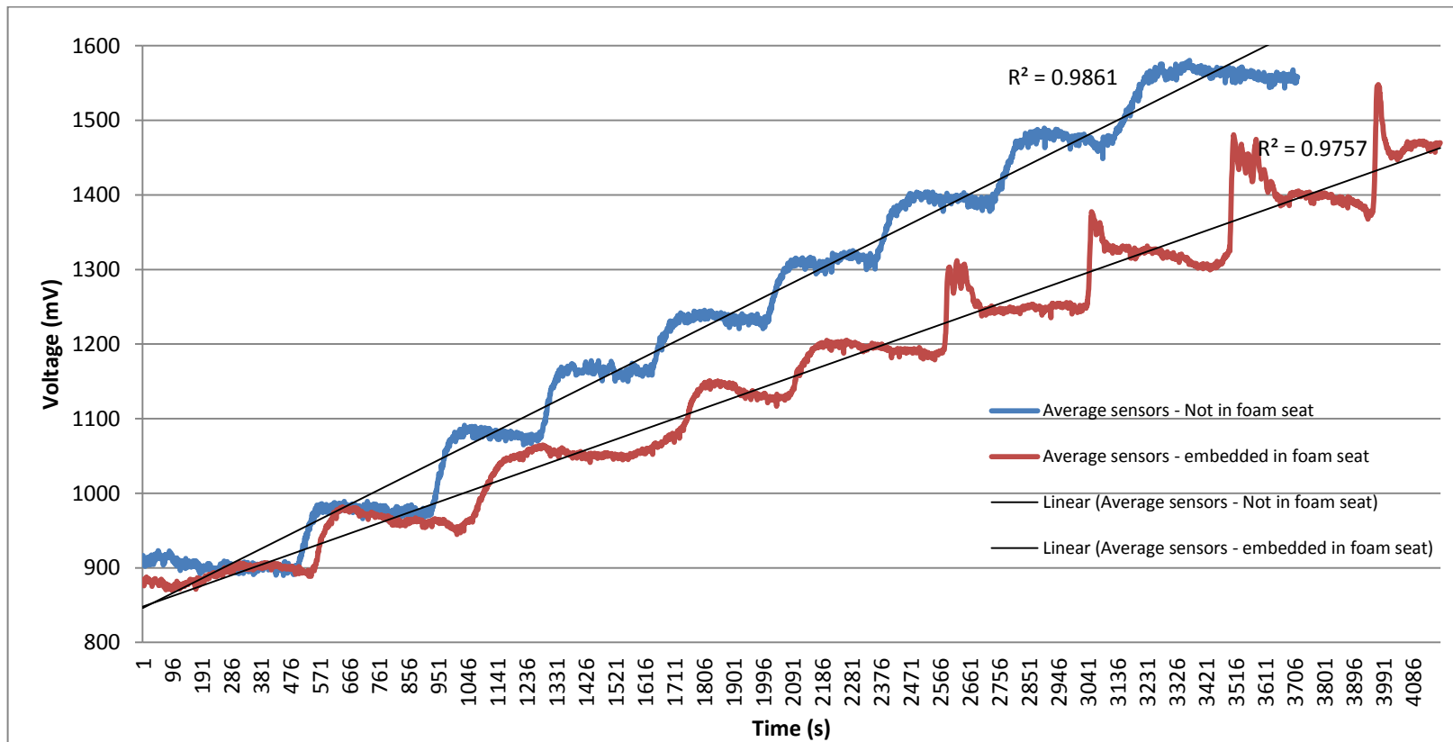
Figure 3.5: The average signals of sensors in two separate conditions when calibrated in the climatic chamber at 25°C between an ascending humidity scale of 30 %RH to 70 %Rh with 5 %RH increments.
