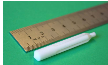
Fig. 4. Manufactured QRFH. (a) Assembly view. (b) Ridge clamped between quarters. (c) Screws along quarter. (d) Bottom of horn, launch-pin’s holes. (e) Dielectric load (cm-ruler).
