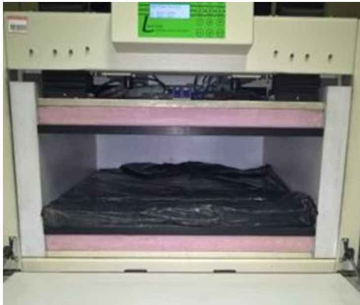
Figure 14: Rigid APM board wrapped in a plastic bag to prevent water vapour adsorption during measurement. Source: Politecnico di Torino.
