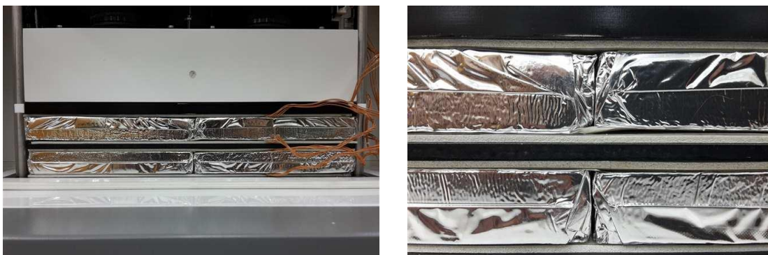
Figure 24: Setup for measurement of \psi values. Source: NTUA – National Technical University of Athens.
