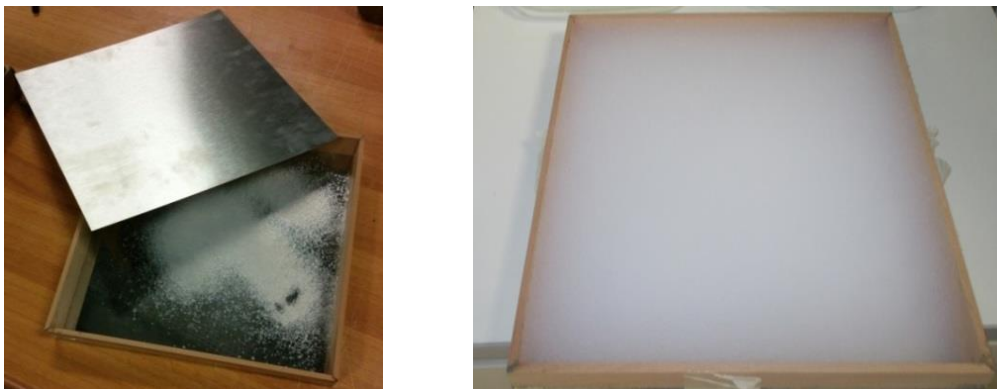
Figure 9: Self-made specimen holder for loose filled granulate made of wooden frame with thin metal plates (thickness of 0.4mm). Source: Università di Perugia.
