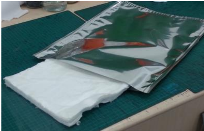
Figure 68: VIP before evacuation.
