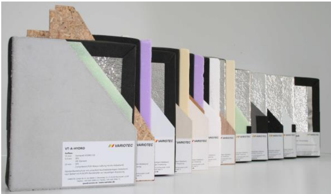
Figure 67: VIP/QASA can be delivered with a number of encapsulation materials.
