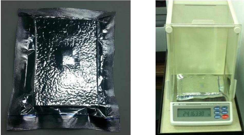
Figure 31: (left) Small panel (~15 cm x 12 cm) with glass fibre and desiccant; (right) weighing the panel with an analytic balance (Shufer, 2017).
