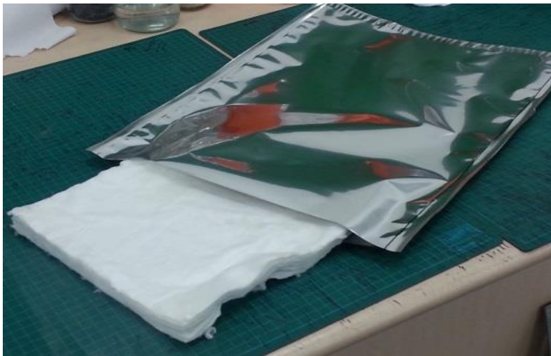
Figure 33: VIP before evacuation.
