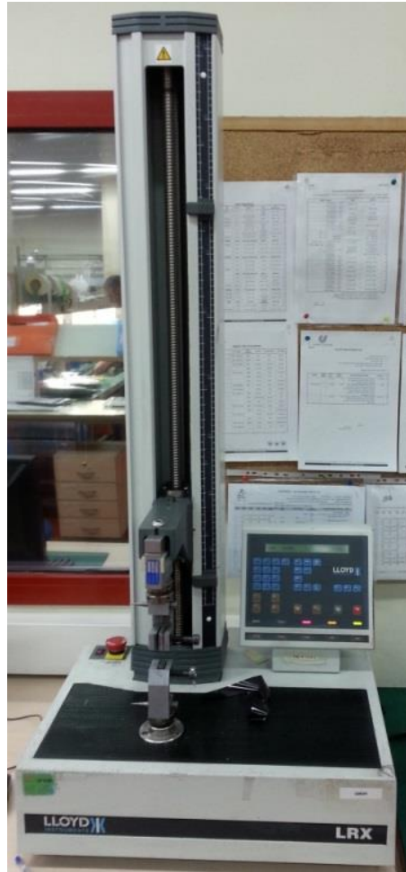
Figure 39: Lloyd Tensiometer as an example unit for testing mechanical properties of VIP envelopes (Shufer, 2017).
