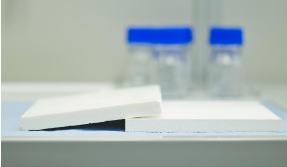
Figure 13: Boards of organic aerogels (polyurethanes) (© BASF).
