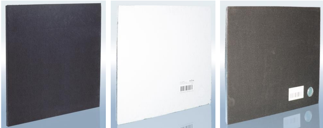
Figure 66: VIP covered by a black glass fibre textile, EPS or rubber granulate lamination.
