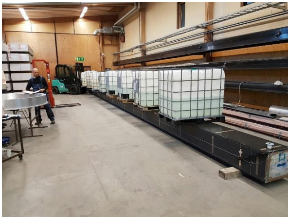
Figure 9. Proof loading of the composite beams during manufacturing, Photo courtesy of Composite Design
