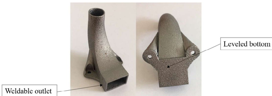
Figure 8. Final propellant flow connector design manufactured with AM LPBF.
